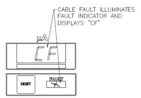
Figure 11: Cable Fault Display
