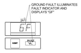
Figure 12: Ground Fault Display
