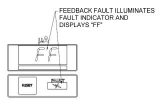
Figure 16: Feedback Fault Display
