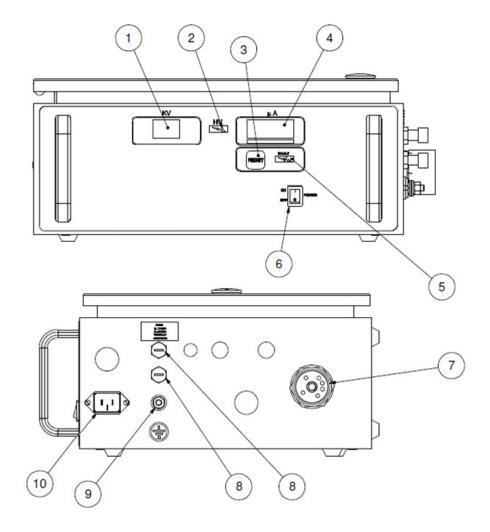
Figure 2: 9060 High Voltage Controller Features (HV2)
