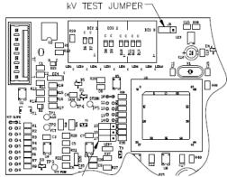
Figure 10: KV Test Jumper Location
