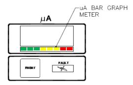
Figure 9: µA Bar Graph Meter Display
