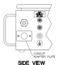
Figure 6: Installation of Conduit Adapter Plate
