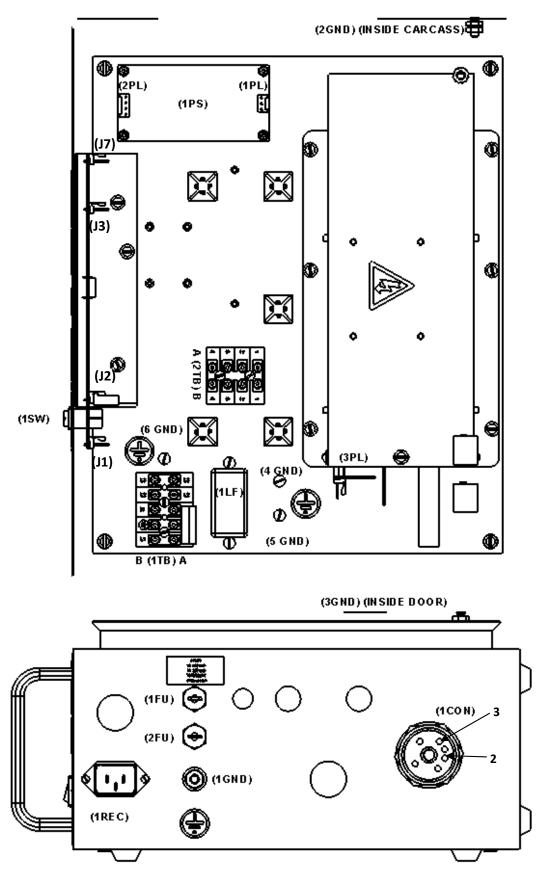
Figure 18: 9060 (80102-21X) Internal Component Locations
