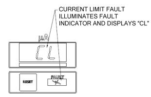
Figure 13: Current Limit Fault Display
