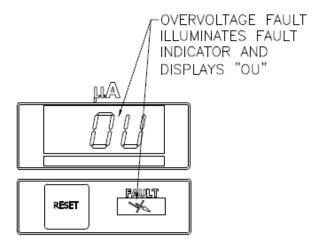
Figure 15: Over Voltage Fault Display
