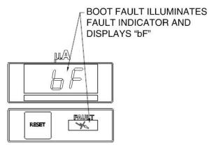
Figure 17: Boot Fault Display
