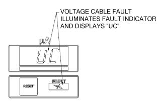
Figure 14: Voltage Cable Fault Display
