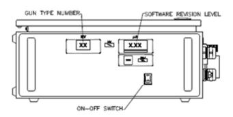
Figure 8: Controller Start-Up Display
